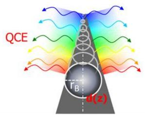
A schematic image of a nanocone-nanowire with a gradually decreasing diameter from Si substrate till the top.
