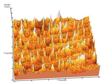
3D AFM image of Ge surface irradiated by Nd:YAG laser at intensity 6.0 MW/cm<sup>2</sup>.
