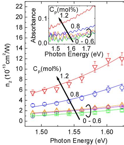
Fig. 4.  $n_2$  spectra of samples with different  $P_2O_5$  concentration ( $C_P$ ). The inset shows the absorption spectra of the same samples.
