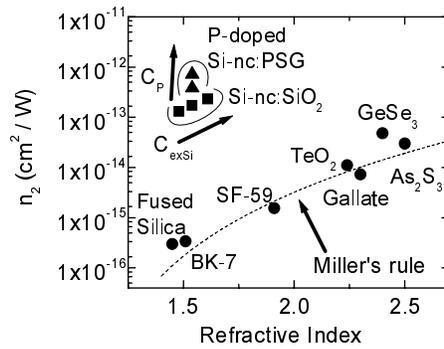
Fig. 5.  $n_2$  is plotted as a function of linear refractive index. The dashed line is the prediction of the Miller's rule. Circles, squares and triangles are the results of several kinds of typical glasses, P-doped Si-ncs embedded in PSG (P-doped Si-nc:PSG) and pure Si-ncs embedded in  $\text{SiO}_2$  (Si-nc:SiO<sub>2</sub>), respectively.
