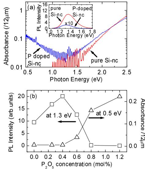
Fig. 1. (a) Absorption spectra of pure and P-doped Si-ncs ( $C_P=0.8\text{mol}\%$ ). The inset shows the PL spectra of the same samples. (b)  $\text{P}_2\text{O}_5$  concentration ( $C_P$ ) dependence of PL intensity at 1.3 eV (Left axis) and absorbance at 0.5 eV (Right axis).
