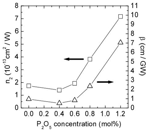
Fig. 3.  $P_2O_5$  concentration dependence of  $n_2$  (left axis) and  $\beta$  (right axis).
