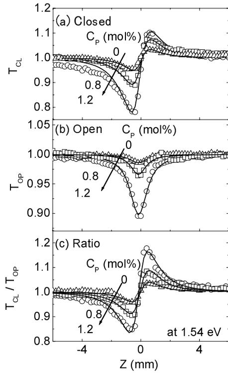
Fig. 2. z-scan measurements for (a) a closed aperture ( $T_{cl}$ ), (b) an open aperture ( $T_{op}$ ) and (c) the ratio of the two results ( $T_{cl}/T_{op}$ ). The squares are experimental results and the solid curves are results of fittings.  $P_2O_5$  concentration ( $C_p$ ) is changed from 0 to 1.2mol% .
